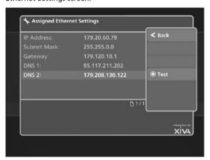
A number of aspects of the connection are tested and reported. If any test fails, check the hint at the bottom of the screen. There are tests whose failure doesn't necessarily indicate a probem with your connection. If the hint suggests it is essential this test passes, please contact your dealer or Imerge Customer Support.
