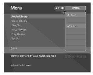
Use the **∧** and **∨** keys on the remote control to step through the options on any screen.
