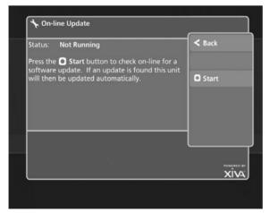
To automatically check on-line for software updates, press the OStart key.
