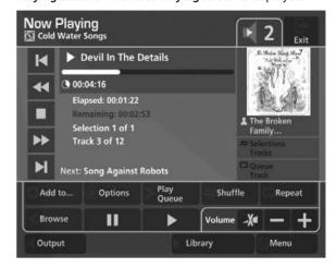
The playback controls appear as buttons on the left hand side of the screen. Touch these buttons to pause, stop, seek or skip through music and movies. The functionality of these controls is explained in more detail on page 25 (audio playback) and page 32 (video playback).
