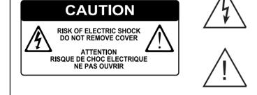
The lightning flash with arrowhead symbol, within an equilateral triangle, is intended to alert the user to the presence of uninsulated "dangerous voltage" within the product's enclosure that may be of sufficient magnitude to constitute a risk of electric shock to persons.
