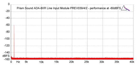
FFT plots made using Prism Sound dScope Series III at 997Hz, 256k points, Prism-7 window, 16 averages, at fs=96kHz, +18dBu=0dBFS line-up level.
