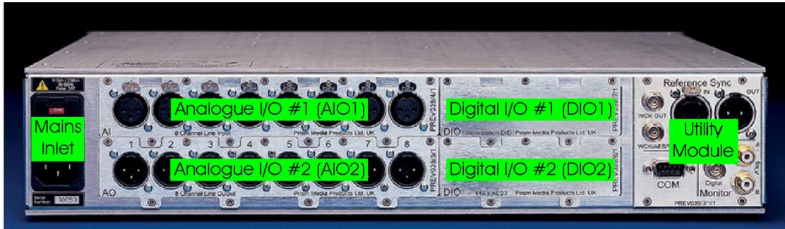
The rear panel of the ADA-8XR is arranged, from left to right when viewed from the rear, as follows:
