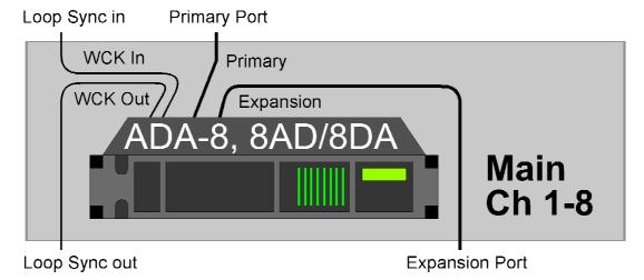
Having connected the ADA-8 as above, switch it on and load the 'Prot HD Main' Store. This is located in Bank 1, Store 1 for ADA-8s without additional digital I/O, and in Bank 3, Store 1 for ADA-8s with additional I/O.
