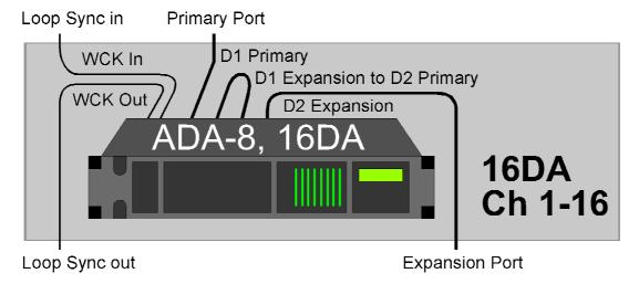
Having connected the ADA-8 as above, switch it on and load the 'ProT HD 2xDAC' Store. This is located in Bank 1, Store 1.
