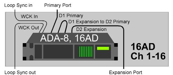
Having connected the ADA-8 as above, switch it on and load the 'ProT HD 2xADC' Store. This is located in Bank 1, Store 1.
