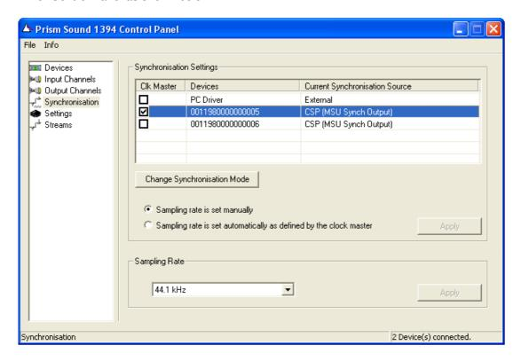
First ensure that the 'Sampling rate is set manually' radio button is selected, as this is the only valid setting for the ADA-8.
