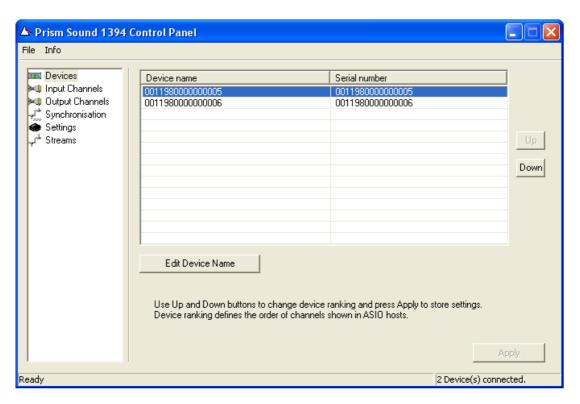
Each ADA-8 device connected to your workstation will appear in the device list, the default name for each device is its GUID. You can find out the GUID of a FireWire I/O Module using the ADA-8 menu system, as described in Section 9.5.3. Note that if your ADA-8 is fitted with two FireWire I/O modules they will both appear in the list as separate devices.
