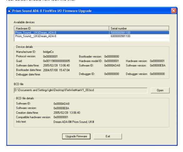
Finally press the 'Upgrade Firmware' button to start the download, the module will automatically restart after the download. Repeat for each module in your system.
