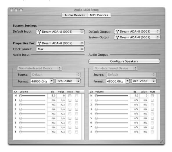
You should also select the ADA-8 unit to be your 'Default Input' and 'Default Output' device using the drop down menus. You may choose to leave the 'System Output' routed to 'Built-in Audio' if you wish.
