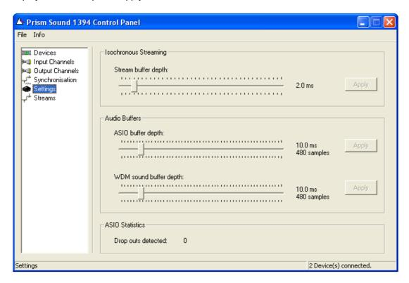
The default setting is 10ms as this gives plenty of margin for reliable operation on the majority of workstations. If you have a requirement for a lower latency you can adjust the buffer depths downwards. You should verify that the new setting works reliably in your environment.
