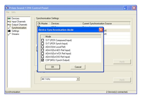
Changes to the synchronization mode of the PC Driver and Device(s) do not take effect until the 'Apply' button is pressed. This is so that changes to multiple devices can take place at the same time.
