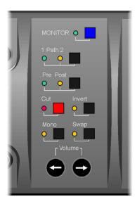
The Monitor Panel controls the ADA-8's two-channel monitor.
