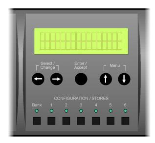
The Menu Panel provides manual control and inspection of all the ADA-8's operating parameters, and also contains the Configuration/Stores buttons for loading and saving setups of the ADA-8.
