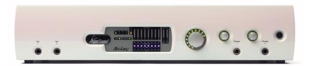
Atlas's front panel contains a limited number of physical controls and indicators. A greater degree of control is available using the <u>Atlas Control Panel app</u> software provided. The front panel also contains the instrument input and headphone output jacks.
