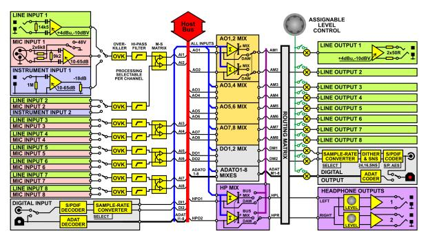
The figure above is a simplified block diagram of the Atlas audio signal paths.
