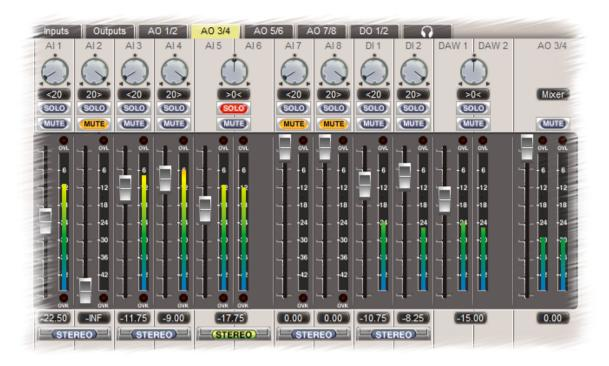
Each input has a fader, a high-resolution <u>peak meter</u>, with overload indication 0.05dB below clipping, plus mute and solo buttons and a pan-pot. By engaging the 'Stereo' button beneath an input pair, the pair is controlled by a single stereo fader, mute button and solo button, and the pan-pots are replaced by a single balance control. The DAW contribution and output strip are always in stereo mode.
