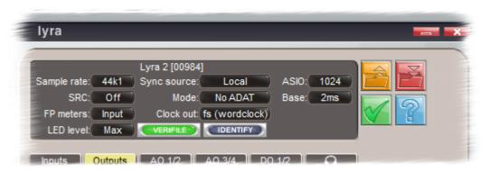
The Lyra model and serial number are displayed at the top of the Unit settings area. Note that the currently-installed firmware version of the Lyra unit can be displayed by hovering the mouse cursor over this text.
