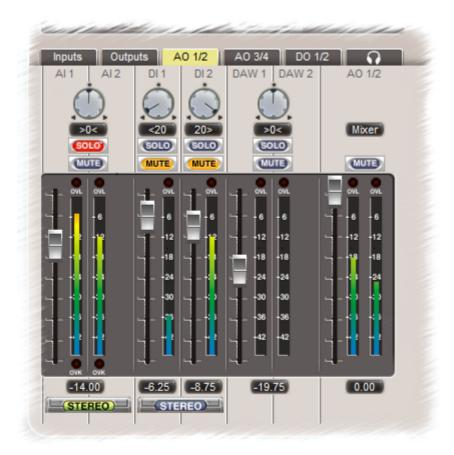
Each input channel has a fader, a high-resolution <u>peak meter</u>, with overload indication 0.05dB below clipping, plus mute and solo buttons and a pan-pot. By engaging the 'Stereo' button beneath an input pair, the pair is controlled by a single stereo fader, mute button and solo button, and the pan-pots are replaced by a single balance control. The DAW contribution and output strip are always in stereo
