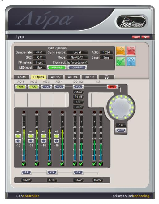
Whilst Lyra can be controlled in a limited way from within the Mac or Windows operating system, or by some audio application programs, most of its detailed features can only be accessed using the Lyra Control Panel app.
