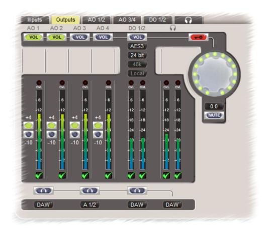
Line output level is switched between +4dBu and -10dBV nominal by the '+4/-10' radio buttons.
