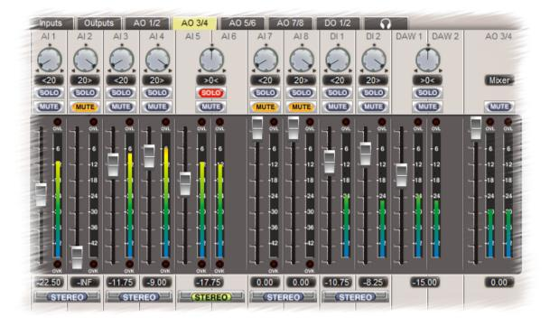
Each input channel has a fader, a high-resolution <u>peak meter</u>, with overload indication 0.05dB below clipping, plus mute and solo buttons and a pan-pot. By engaging the 'Stereo' button beneath an input pair, the pair is controlled by a single stereo fader, mute button and solo button, and the pan-pots are replaced by a single balance control. The DAW contribution and output strip are always in stereo mode.
