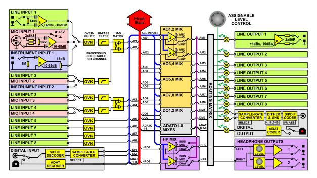
The figure above is a simplified block diagram of the Titan audio signal paths.
