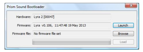
This displays the type of device and its serial number, along with the version and timestamp of the currently installed firmware.
