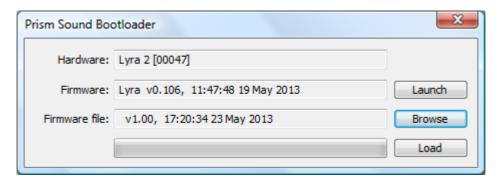
At this point, a warning may be issued if the selected firmware file is older than the firmware currently installed in the unit.
