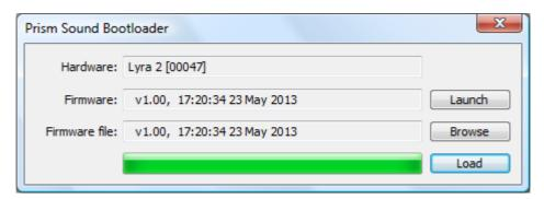
Finally click the 'Launch' button, which will cause the unit to reboot with the new firmware installed.
