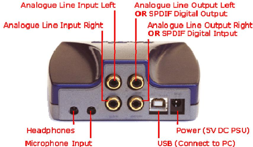
Your BB2 should come with a USB2 (A to B) cable, and a 5V DC power supply (PSU), with a mains plug appropriate to your geographical location.
