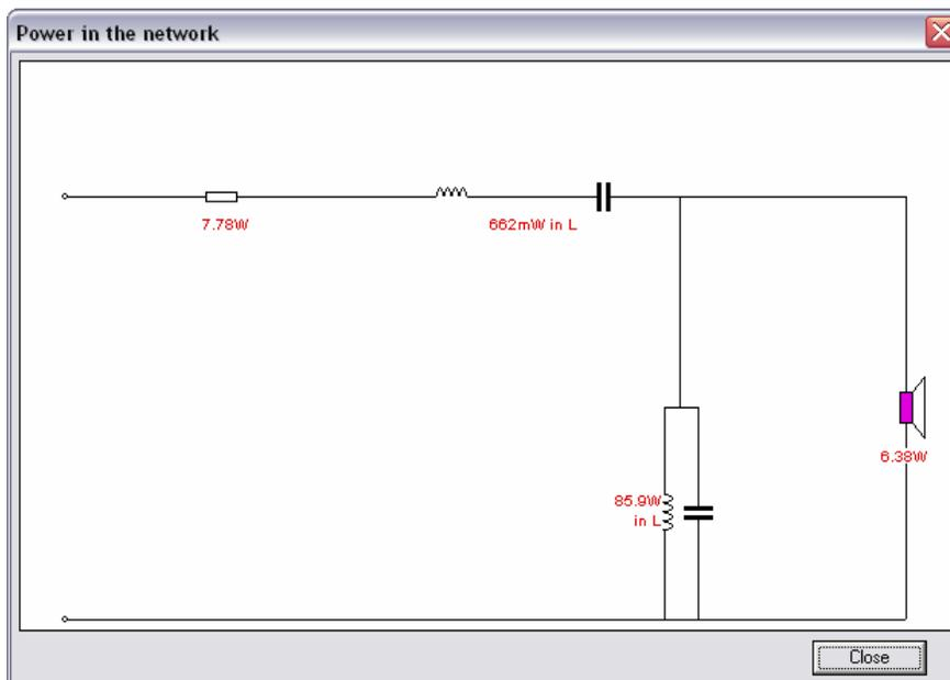
Figure 13. Real Power in 3-way section 2 (Midrange)
