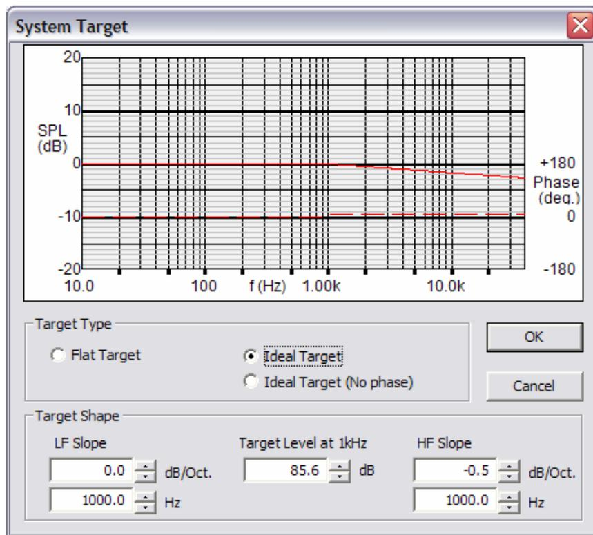
Figure 21 System target
