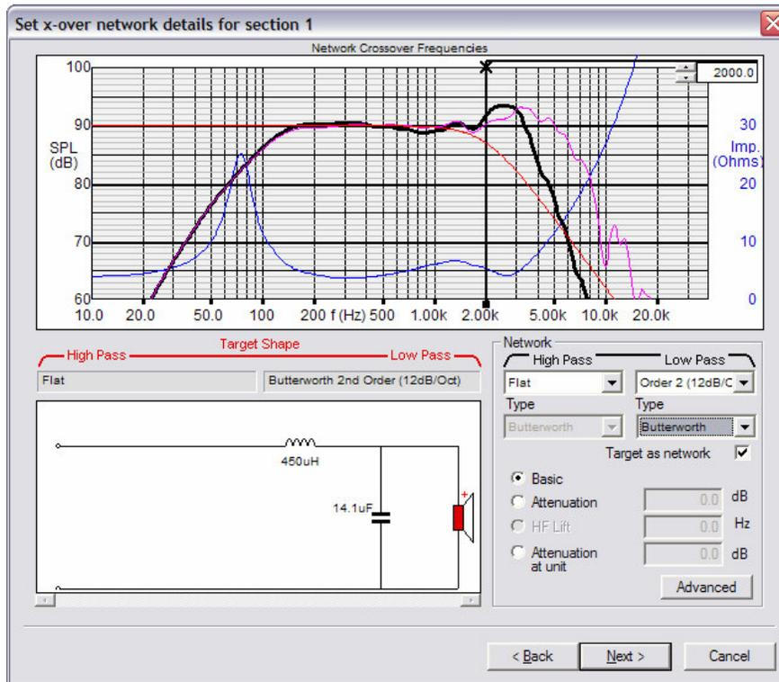
Figure 4. X-over type and target response
