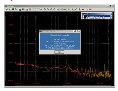
Either track 41 or track 42 should result in complete cancallation of the signals. If this is the case, then Downmix has been implemented correctly.
