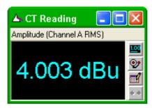
Within a Reading are the result itself, its units, and settings for the name of the Reading, the number of decimal places to display the result, limit values to check against, etc. Auto Sequence uses these settings to determine if and how the measurement should be limit checked and how the result should be displayed in the report.
