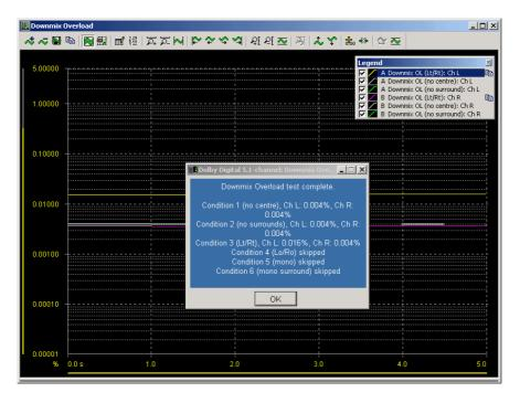
The distortion should be less than 3% THD+N for all conditions measured.
