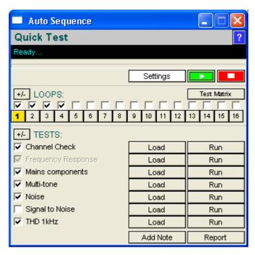
In this example, there are 16 Loop files defined in the folder and there are consequently 16 corresponding Loop buttons and check boxes. Entire Loops can be disabled using the Loop check boxes in which case they will not be run and will not be required for the pass/fail. The interface will support up to 48 Loops which would give three rows of Loop buttons.
