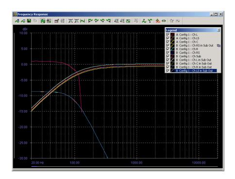
For Test 2, the Left and Right outputs will show a flat frequency response with no redirected bass present at the Sub output.
