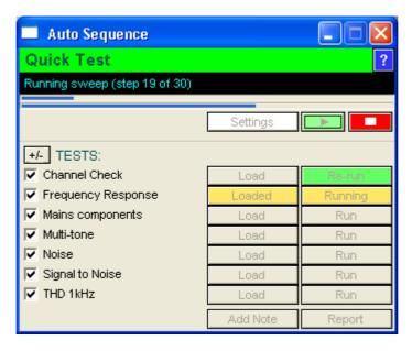
In the above screen-shot, the header bar tells us the name of the Test Sequence and is coloured according to whether the overall Test Sequence is passing or failing. If it is passing (as above) this will be green. It will be red for failure and it will be remain grey if there is no limit checking encountered. The status bar below this tells us what Auto Sequence is currently doing ("Running Sweep: (step 19 of 30)" in this case...").
