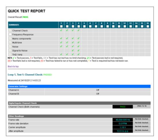
HTML reports work in two "modes" depending on whether the option to "Save a new report for every Test" is checked. (Settings menu). If this is checked (default), every time the Test Sequence is run, it will create uniquely named HTML reports and graphics. The name is made up of the serial number/reference (if entered), the date and time of the report, and an indicator of pass (P) or fail (F).
