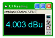
They are created by clicking on the measurement result in one of the analyzer windows and dragging it out onto the page. Once created, click on the buttons on the right to configure the Reading. Please see the dScope Series III Operation manual for further information on creating and using Readings.
