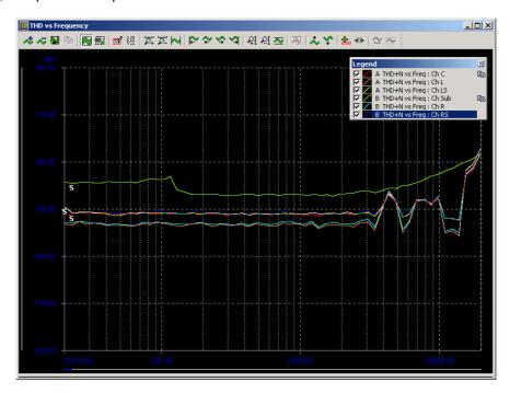
Across the frequency range, the THD+N for line outputs should be less than –60dBr and for headphone or speaker outputs, less than –57dBr. At higher frequencies, it is usual to see an increase in distortion.
