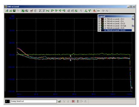
Across the amplitude range, the THD+N for line outputs should be less than –60dBr and for headphone or speaker outputs, less than –57dBr. Typically, the THD+N will decrease slightly for the first 10 or 20dB and then reach a low, constant level.
