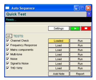
This is an alphabetical list of the Configurations found in the selected folder. To the left are check boxes to set which Tests will be run in the sequence. To the right are buttons to manually load the Configuration and to run the Tests contained in it. If the [Run] button for a particular Test is clicked, it will first load the associated Configuration if it isn't already loaded then run the Test.
