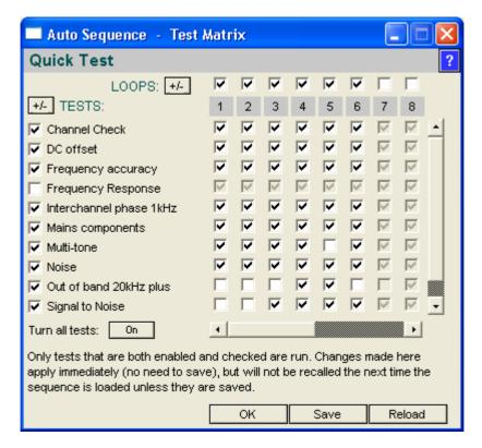
Here, only the Tests that are both enabled *and* checked will be performed and are required for the pass/fail results.
