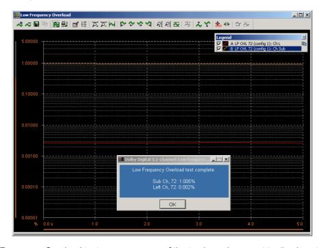
If the Low Frequency Overload test passes on one of the tracks, subsequent testing is not necessary. The script will detect this and will only prompt for the next track if the previous track caused the overload test to fail.
