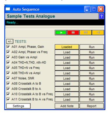
This is an alphabetical list of the Configurations found in the selected folder. To the left are check boxes to set which Tests will be run in the sequence. To the right are buttons to manually load the Configuration and to run the Tests contained in it. If the [Run] button for a particular Test is clicked, it will first load the associated Configuration if it isn't already loaded then run the Test.
