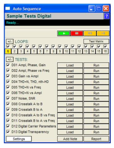
In this example, there are 16 Loop files defined in the folder and there are consequently 16 corresponding Loop buttons and check boxes. Entire Loops can be disabled using the Loop check boxes in which case they will not be run and will not be required for the pass/fail. The interface will support up to 48 Loops which would give three rows of Loop buttons.
