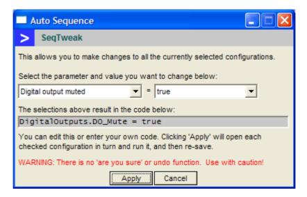
The idea here is that you select the parameter you want to change, the value you want to change it to, and Auto Sequence will make the changes to all the currently selected Configurations by sequentially opening each one, running a line of script code and then re-saving the configuration.
