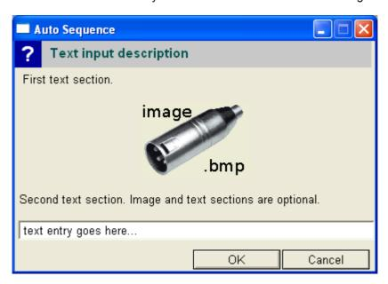
If [OK] is clicked the entered text is included in the results and the Sequence continues. There is no limit checking, but the text field cannot be left empty. If a blank entry is required, a space character can be entered, or some other entry such as "None" or "N/A".
