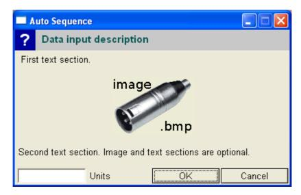
The form *requires* a numeric input in the edit box at the bottom left, but this doesn't have to be limit checked. The "Units" text is a user defined text string.
