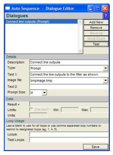
The list box at the top displays the list of Dialogues defined for this test. They are executed in the order shown. Dialogues can be added, removed, moved up or down and tested using the buttons to the right of the list. The [Test] button runs the highlighted Dialogue to check its function (preview dialogues and/or check logic)
