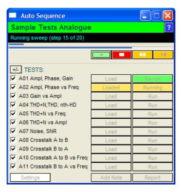
In the above screen-shot, the header bar tells us the name of the Test Sequence and is coloured according to whether the overall Test Sequence is passing or failing. If it is passing (as above) this will be green. It will be red for failure and it will be remain grey if there is no limit checking encountered. The status bar below this tells us what Auto Sequence is currently doing ("Running Sweep: (step 15 of 20)" in this case...").
