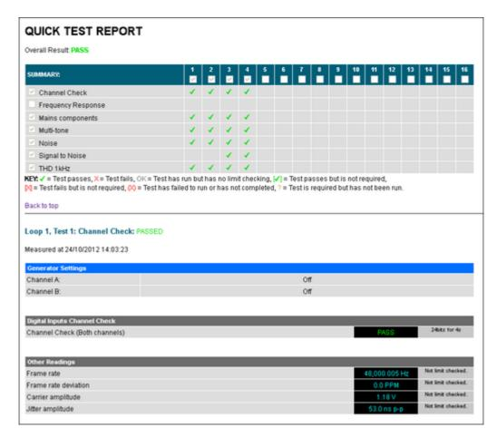
HTML reports work in two "modes" depending on whether the option to "Save a new report for every Test" is checked. (Settings menu). If this is checked (default), every time the Test Sequence is run, it will create uniquely named HTML reports and graphics. The name is made up of the serial number/reference (if entered), the date and time of the report, and an indicator of pass (P) or fail (F).
