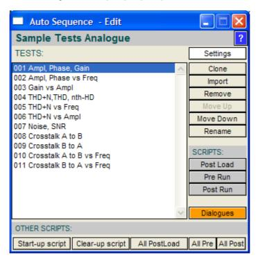
The [Settings] button provides access to the same <u>settings controls</u> as the [Settings] button on the Sequence dialogue.
