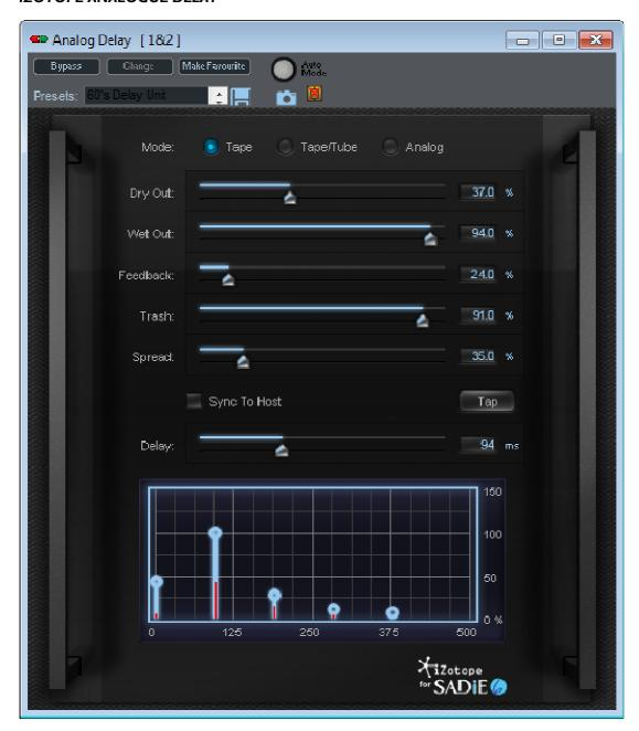
The **Analog Delay** process is of course not an analogue process, but is digitally modelled to allow you add analogue and tape-style echoes to your tracks. This vintage gear-inspired delay unit has unique features, including a delay meter that lets you see and adjust the level and spacing of each echo generated.
