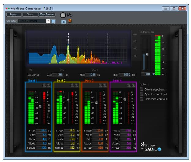
The Multiband Compressor gives you complete control over the dynamic range of your audio. It features a crossover, which allows you to adjust the dynamics of four frequency bands independently.
