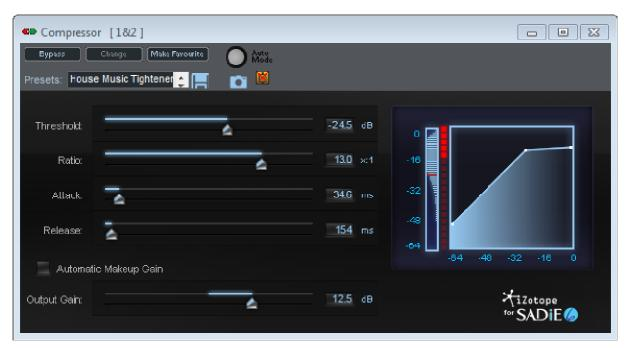
The Singleband Compressor gives you control over the dynamic range of your audio. It features a meter to show the compression curve, as well as how it is affecting the audio.
