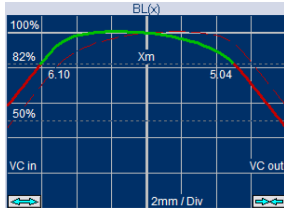
The BL( x ) curve shows how BL is varying with in/out excursion ( x ) of the Voice Coil
