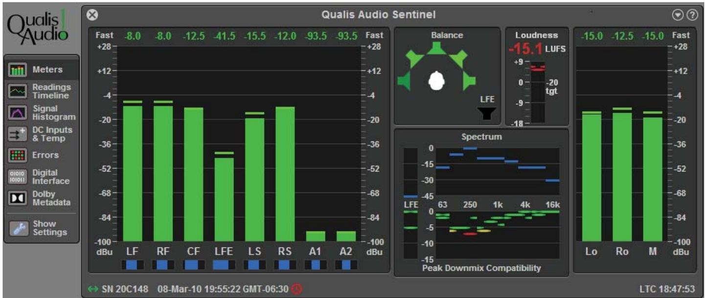
The Qualis Audio SENTINEL takes a different approach. It *directly* assesses stereo and mono compatibility of a surround mix. The measurements are converted to a set of numerical results indicating the amount of signal lost by downmixing as a function of frequency. These values may be tested and error conditions may trigger an alarm. The user is freed from watching and interpreting a screen, allowing attention to be given elsewhere where it may be needed more.
